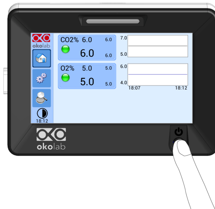
Figure 74. How to enter in Touch Screen Calibration.
